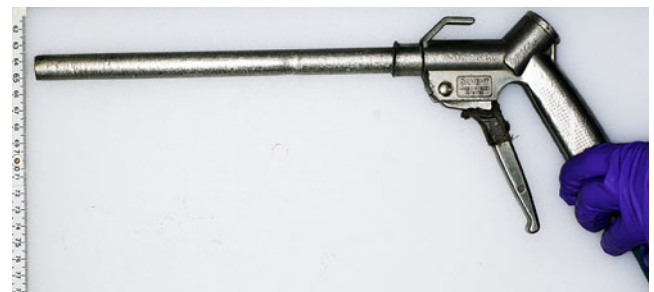
Fig. 4 The nozzle of the compressed air cleaner has a diameter of about 12 mm and is connected to a stationary air pressure system via flexible hose
